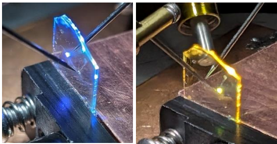
Fig. 1. Real-color electroluminescence images obtained for the double-sided sample with LED structures grown on both sides. The images were captured under positive bias applied to the (a) Ga-polar and (b) N-polar surfaces, each emitting at different wavelengths due to the varying chemical compositions of the grown active regions.
